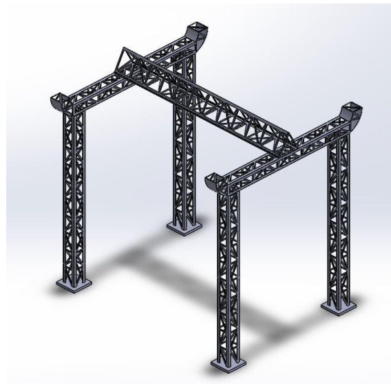
Figure 1.3D model of mast crane in Solidworks
